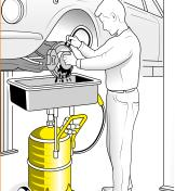
Washing with brush with continuous liquid flow
