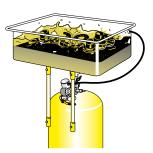
Dip washing with parts placed in the tank
